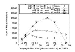
Fig. 6. Breakup of Number of Retransmissions for 802.11
