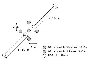
Fig. 1. Field Topology - 5 Bluetooth nodes, 4 802.11 nodes. Bluetooth devices have RIA.
